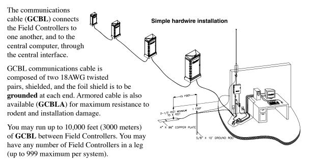
A chain of controllers connected by the communications cable (GCBL) is called a "leg". Two separate legs can be wired from the central interface to the field.
