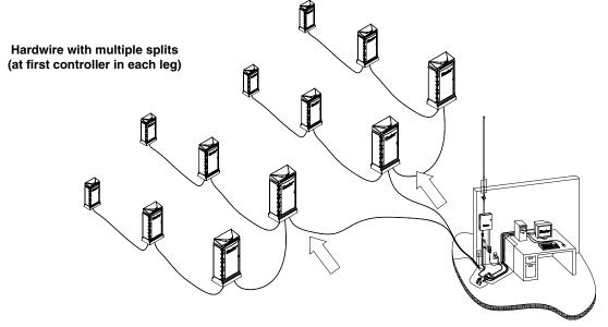
You can also "split" either (or both) of the legs at the first Field Controller in a leg. This allows the most cost-effective route to each Field Controller, by allowing the four shortest possible wire runs. The communications is split at the terminal strip, on the hardwire communications board inside the Field Controller – *never splice the cable itself*.
